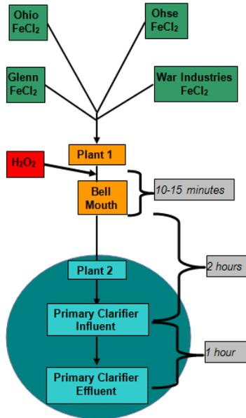
Figure 1. Schematic of Plant 1 to Plant 2 Chemical Odor Control
