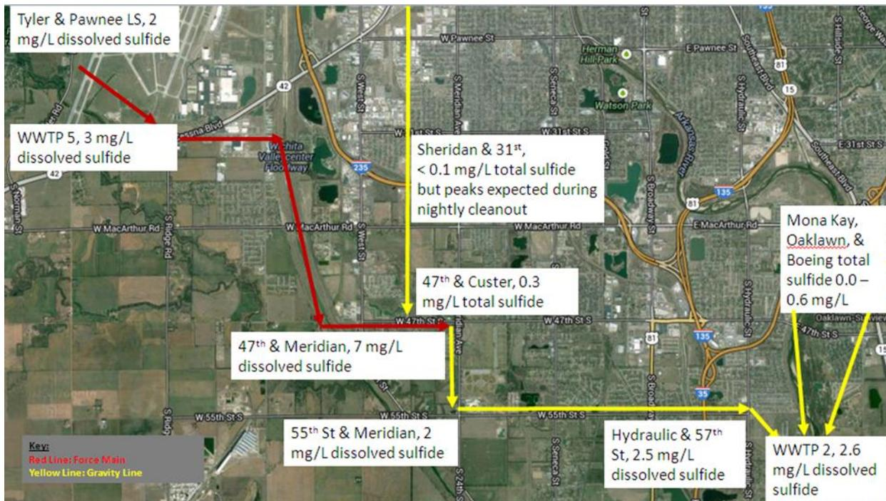
Figure 2. Diagram of Major Plant 2 Forcemains and Interceptors (Plant 1 Flows Not Shown)
