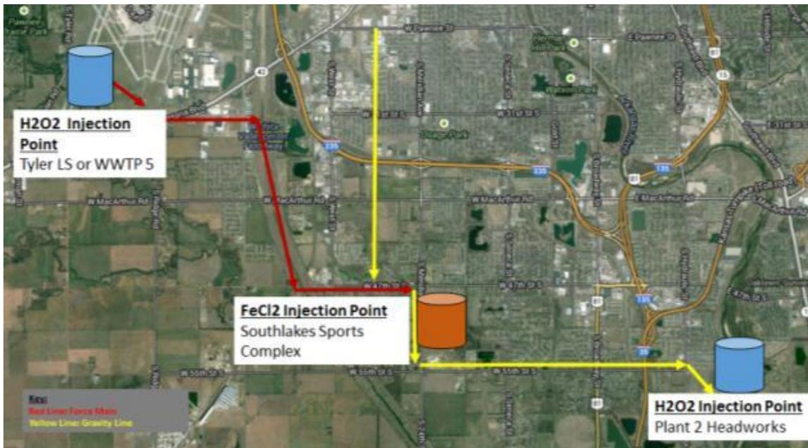
Figure 3. Plant 2 Collection System Proposed Chemical Dosing Sites
