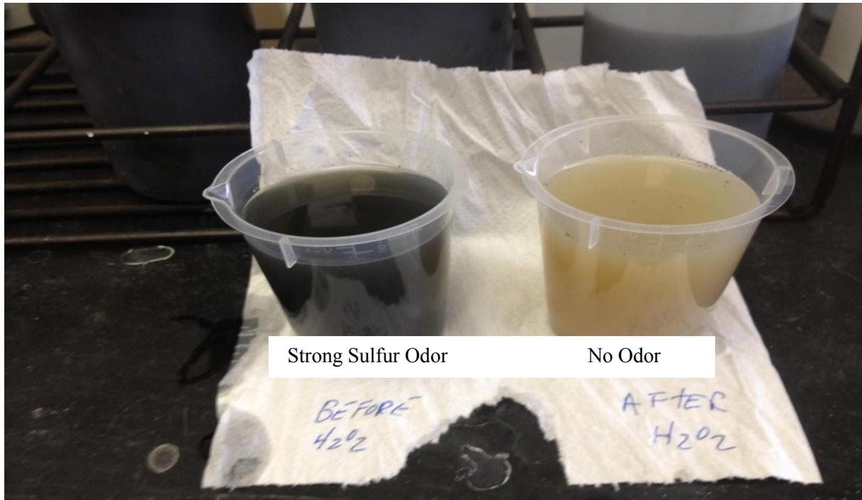
**Figure 6. Direct Oxidation of RSC in Wastewater with H<sub>2</sub>O<sub>2</sub>**
