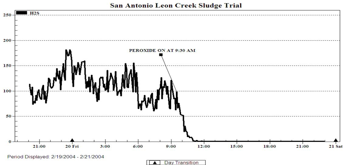
Additional testing of the gas phase on DAFT #3 was performed to verify the long term suppression of hydrogen sulfide generation during the period of February 21 through February 27 (Figure 2). All results with the exception of two periods when the feed system was shut off showed below detectable levels.
