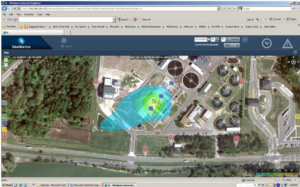
**Figure 3. OdoWatch System at HRSD CETP**
