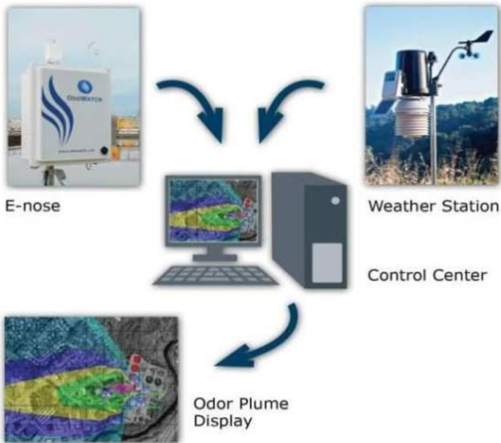
**Figure 2. OdoWatch Odor Monitoring System**
