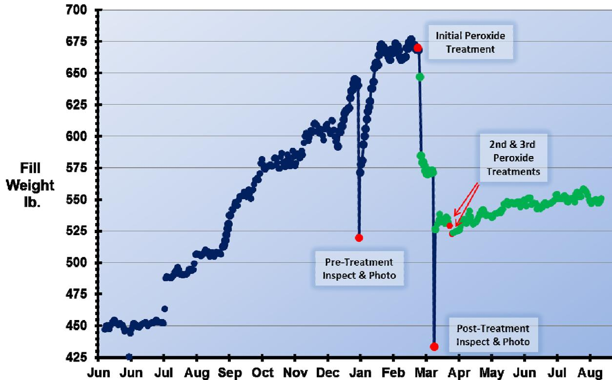
Figure 37. On-line fill pack weight measurements from installation through peroxide cleaning. The initial peroxide cleaning removed 150 lb. of deposit weight from the test cell.
