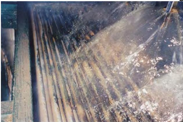
**Figure 14. Tube bundle showing some bare tube metal part way through the cleaning procedure.**
