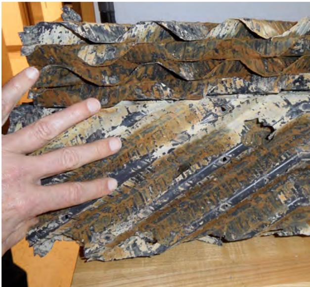
**Figure 21. Close up of cross-fluted fill 7 months after restoring proper treatment**
